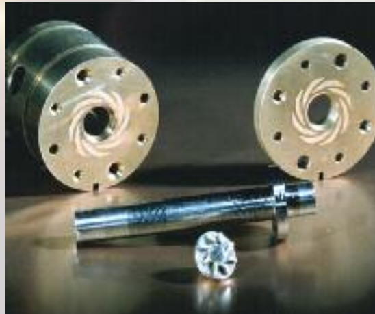
Herringbone journals, inward pumping thrust plates 400,000 rpm cryogenic helium gas lubricant
